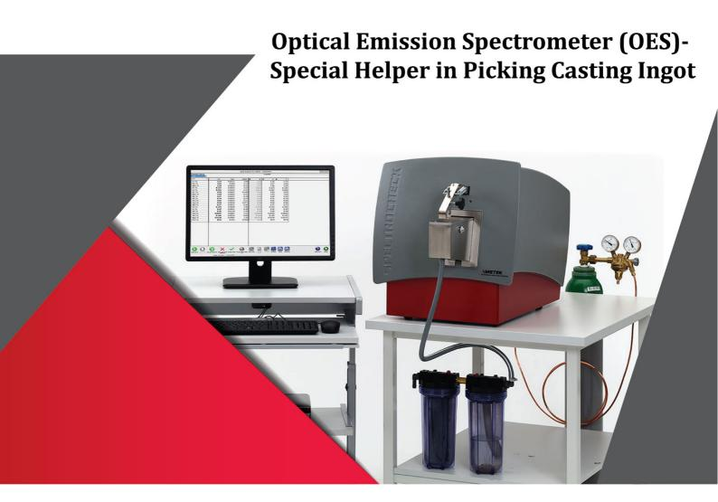
Failure in compliance to chemical composition of alloyed aluminum may result in brittleness of the casting part. Thus, before reaching the furnace, it's an essential first step to test the chemical composition of the raw material.
